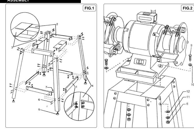
Before you begin, separate all parts and group by size and style. If any parts are missing, contact your Sealey stockist immediately. **NOTE**: finger tighten nuts and bolts when assembling. Once assembled, use an adjustable wrench to ensure all fixings are secure. **WARNING!** This stand must be installed on solid level ground and in combination with compatible bench grinders.
